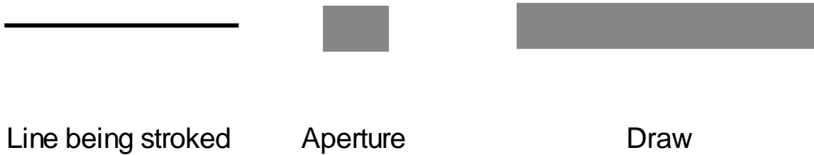
1. Creating a draw: the aperture is aligned with line
